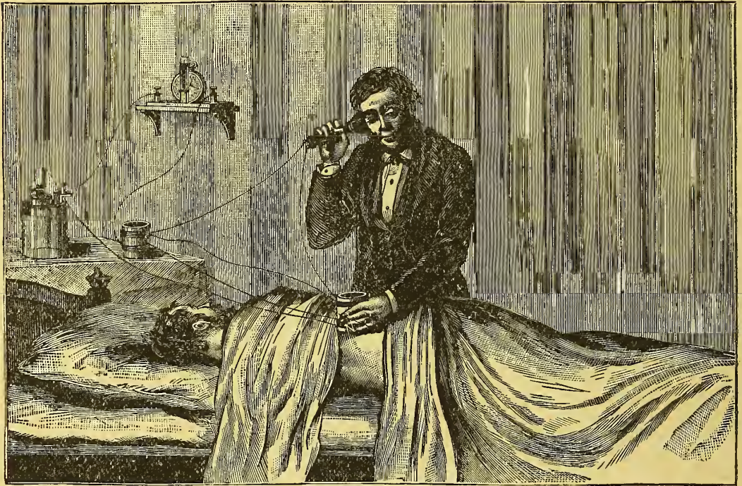
Fig. 5.—SEARCHING FOR A HIDDEN BULLET BY THE INDUCTION BALANCE.
